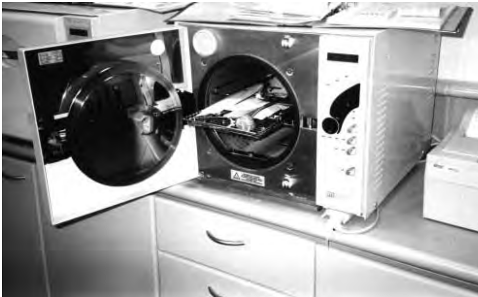
The autoclave is used to sterilise dental instruments, an important stage of effective infection control.
