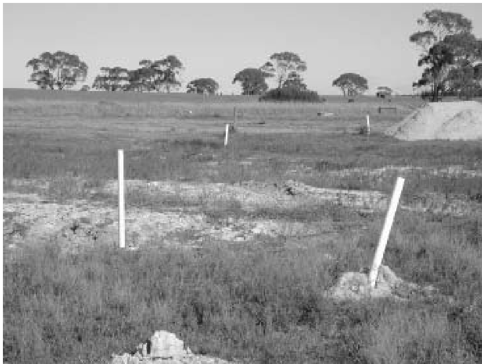
Part of the network of monitoring bores on the site.
