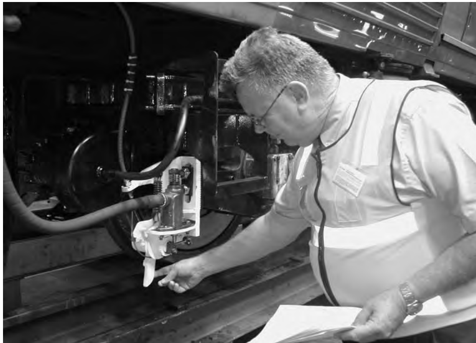
DoI safety auditor inspecting a train braking mechanism.
