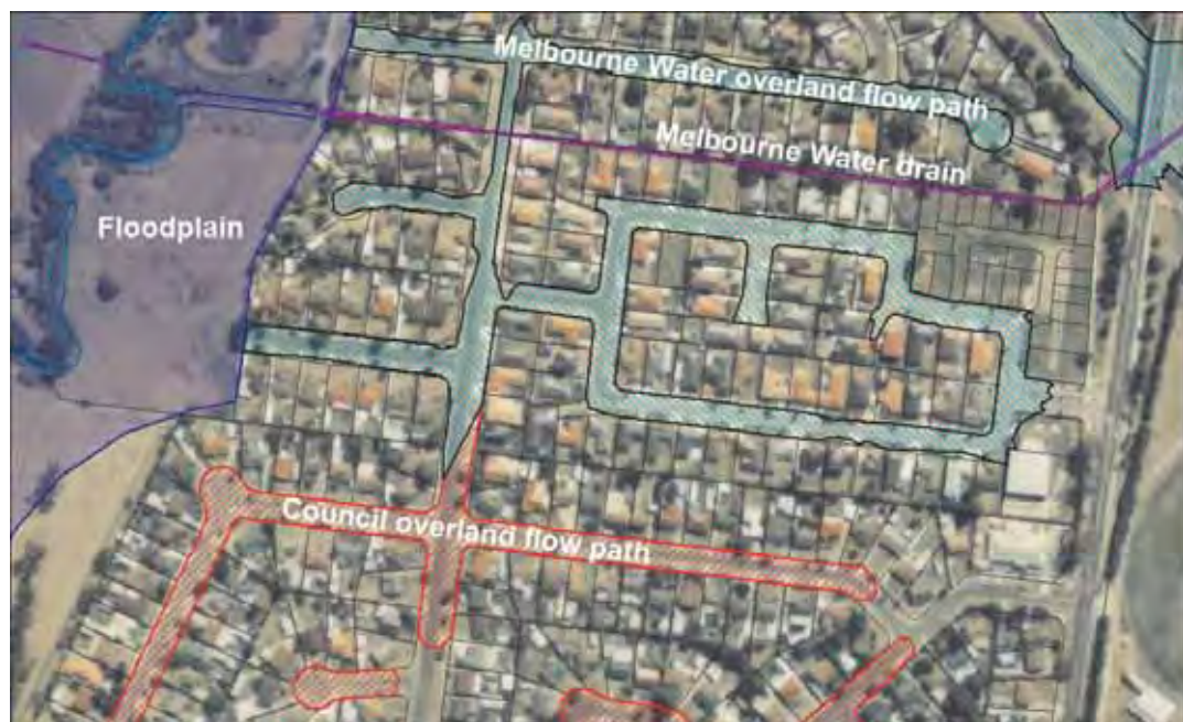
Impact of large storm event on new suburb.
